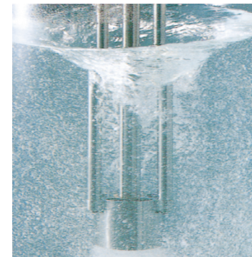
Liquid flow in reverse operation(optional)
